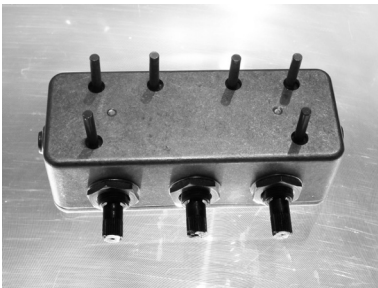
Fig. 3 The bi-core unit, left potentiometer controls on-time of the LED, right potentiometer the off-time.
