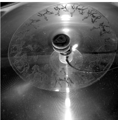
Fig. 4 The Picture-disc is mounted on a dc-motor. The motor is fixated with vacuum cup on the screen.
